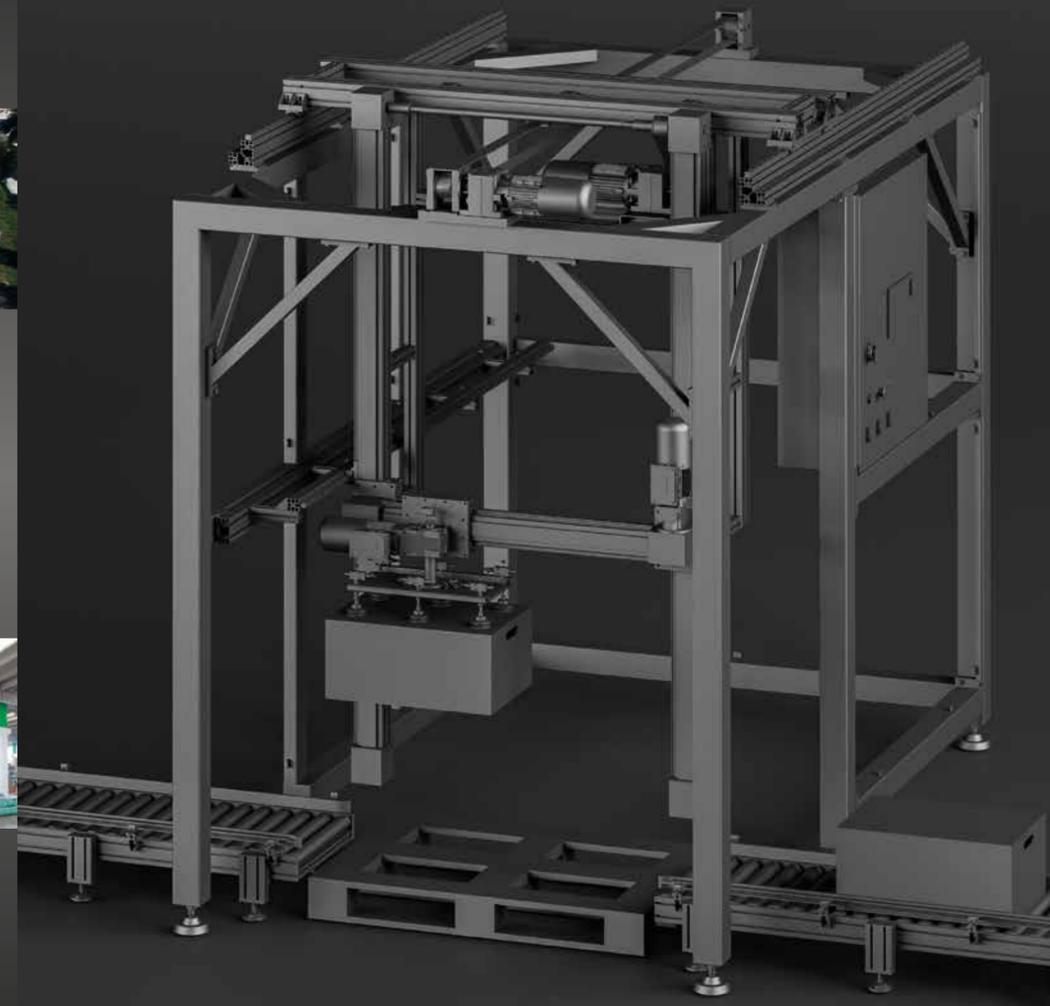
The 4-axis Robot Palletiser is a compact and reliable solution with a small footprint and a 360° working area. It can work on several palletising or depalletising lines at the same time, and by using a single pick-up gripper it guarantees the required capacity and is able to meet **multiple layout requirements**.
